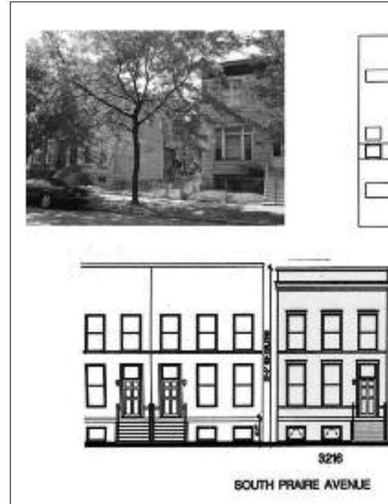
Submittal materials for proposed new construction projects should include a street-view photo, a block site plan, and a streetscape elevation showing the proposed new infill.
